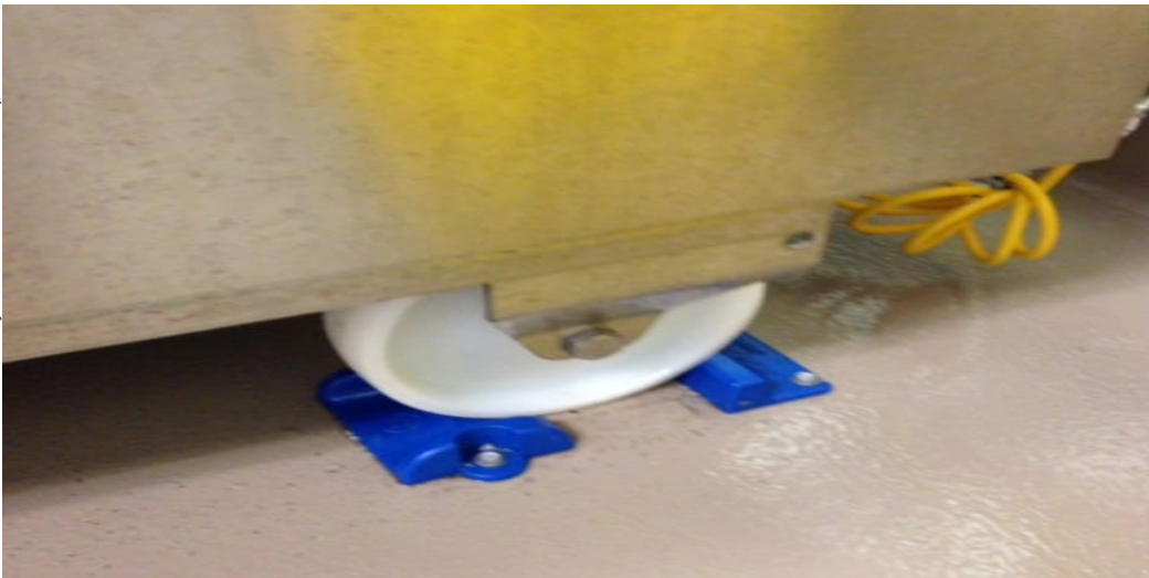
A chock system such as the one shown here can help kitchen staff ensure that cooking appliances moved for cleaning are put back in the right spot.
